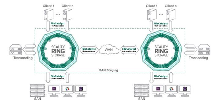
FileCatalyst enables remote users to transfer data to and from remote sites at high speeds and provides reliable data transfers between geographically distributed Scality RING infrastructures.
