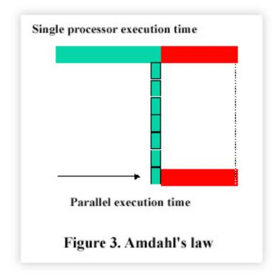
Figure 3 attempts to show this effect more intuitively. The parallel portion of the total execution time can he reduced in proportion to the number of processors applied to the workload. The serial portion, however, remains unchanged since only a single processor can perform that work. As more and more processors are added to increase the degree of parallelism, the fixed serial portion dominates the reduced execution time and is responsible for the sublinear "bending" in the scale-up curve.
